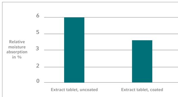
Moisture barrier test (duration 1 week). The extract tablet core was coated with NutraPolish® Organic (5% weight gain) and absorbed less water than the uncoated extract core.
